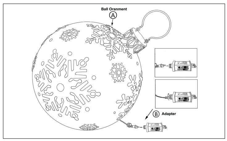
1. Connect the transformer (B) to the figure (A).
